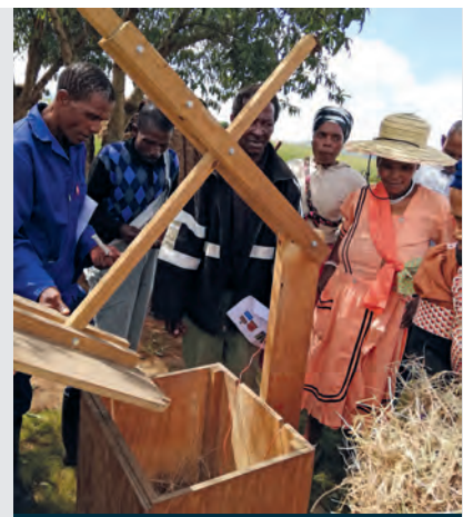
This hay baler was custom made by the Institute of Natural Resources (INR).
