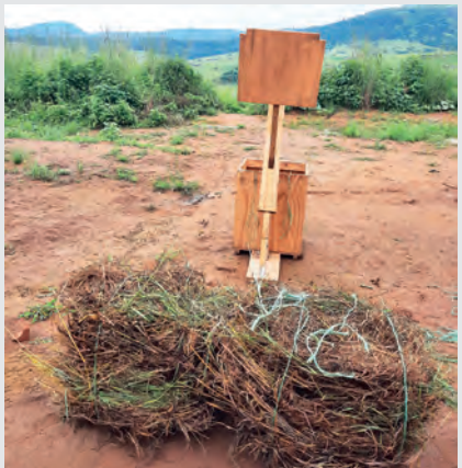
Small scale farmers from the Mahlathini Development Foundation in Bergville use a hand-operated hay baler to preserve veld grass for their livestock. Their baler was custom-made by the Institute of Natural Resources. The baling box is attached to a platform to provide stability and to balance the lever arm. Baling rope is placed inside the box prior to filling it with straw. Once the box is full and the loose straw is compacted, the bale is tied, removed from the box, and stored.
