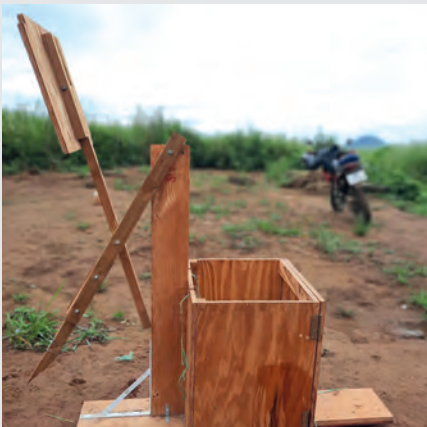
Small scale farmers from the Mahlathini Development Foundation in Bergville use a hand-operated hay baler to preserve veld grass for their livestock. Their baler was custom-made by the Institute of Natural Resources. The baling box is attached to a platform to provide stability and to balance the lever arm. Baling rope is placed inside the box prior to filling it with straw. Once the box is full and the loose straw is compacted, the bale is tied, removed from the box, and stored.
