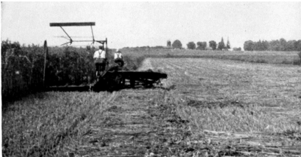
In the northern part of the Corn Belt the hemp usually does not grow so tall and therefore can be handled more easily with machines. During the first World War hemp-harvesting machinery was developed. These harvesters (see above) in one operation cut
