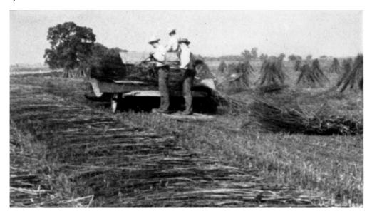
The most efficient method is to use the pick-up binder. These machines, drawn by tractors, cover about an acre an hour. They pick up the retted hemp stalks and tie them into bundles in one operation. The machines are part of the modern hemp-mill equipment and are rented to farmers.
